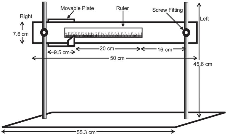
FIG. 2. Back view of the Müller-Lyer apparatus, showing the measuring scale with markings in mm.
