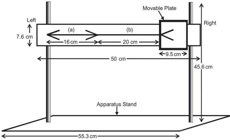
FIG. 1. Front view of the Müller-Lyer apparatus, showing the fixed line on the left and movable or variable line on the right.
